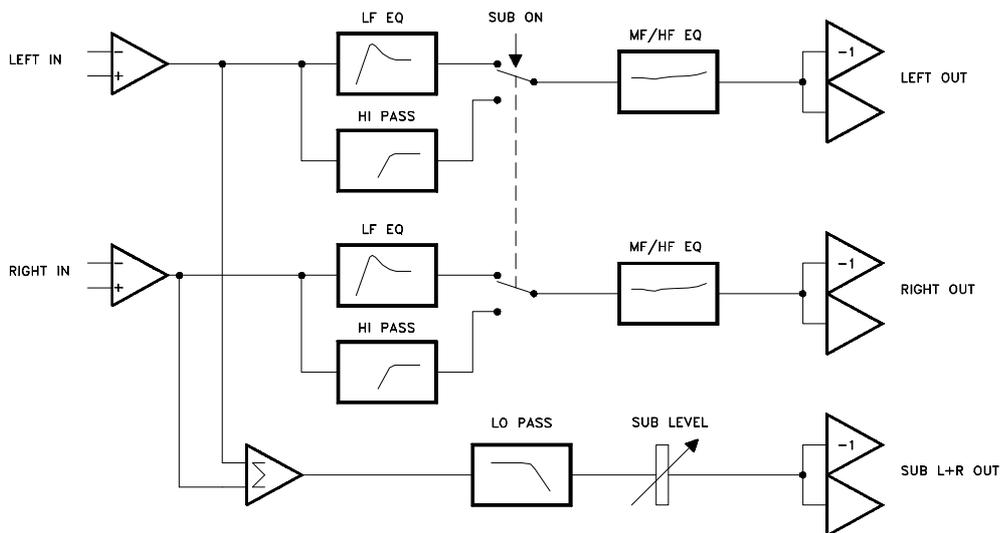
**Figure 4. TX1 simplified block diagram.**
