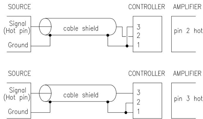
**Figure 2. Input connections from an unbalanced source**
