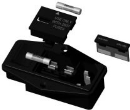
Fig. 3. IEC input module showing fuse location and input voltage selector orientated for insertion at 200V - 240V usage.
